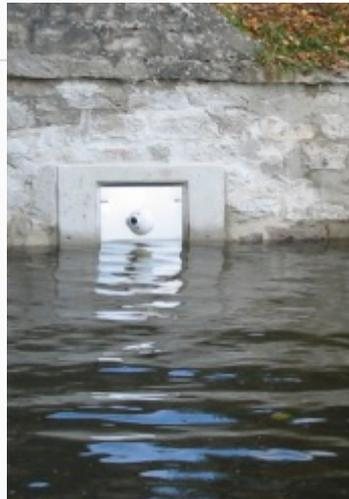
**Flow measurement using the hemisphere sensors**
