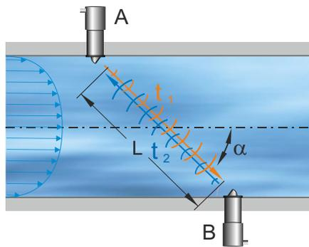
The NivuFlow 650 measurement principle is based on detecting the transit time of ultrasonic signals between two sensors (A and B).
